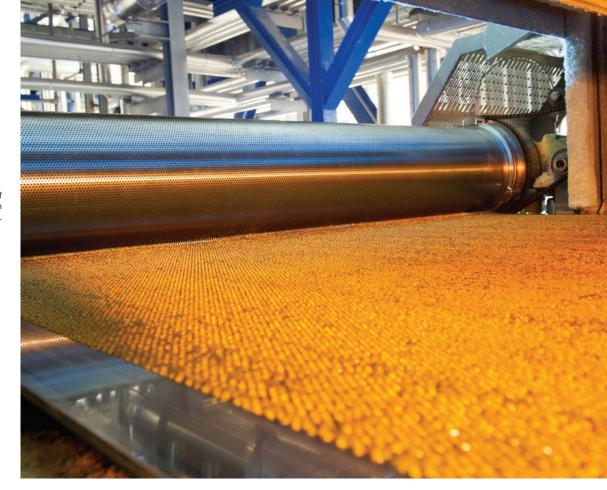
Discharge of sulphur pastilles from steel belt cooler.
